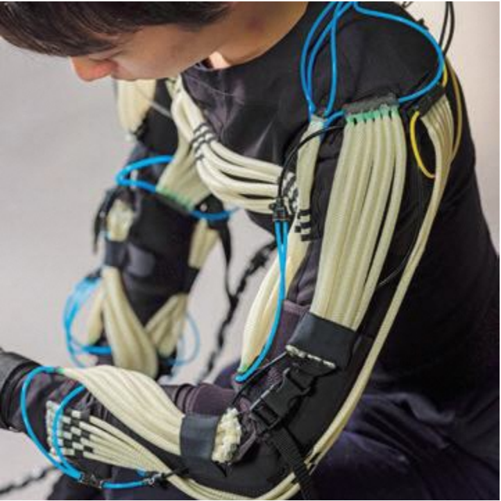
An example of a power support suit operated by artificial muscles
