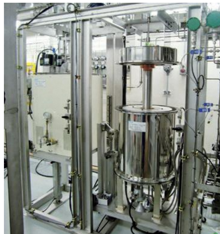
Measurement device of thermal properties of hydrogen
