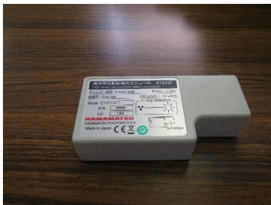
Image 5: High-dose-rate CsI detector (Hamamatsu Photonics K.K. C12137)
