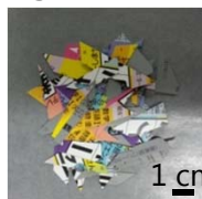
Magnetic card (PET+Fe, Ti, Al)
